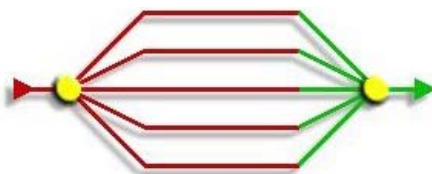
Fig. 2. The schematics of a memory with 5 channels and selection valves (the light grey circles)
